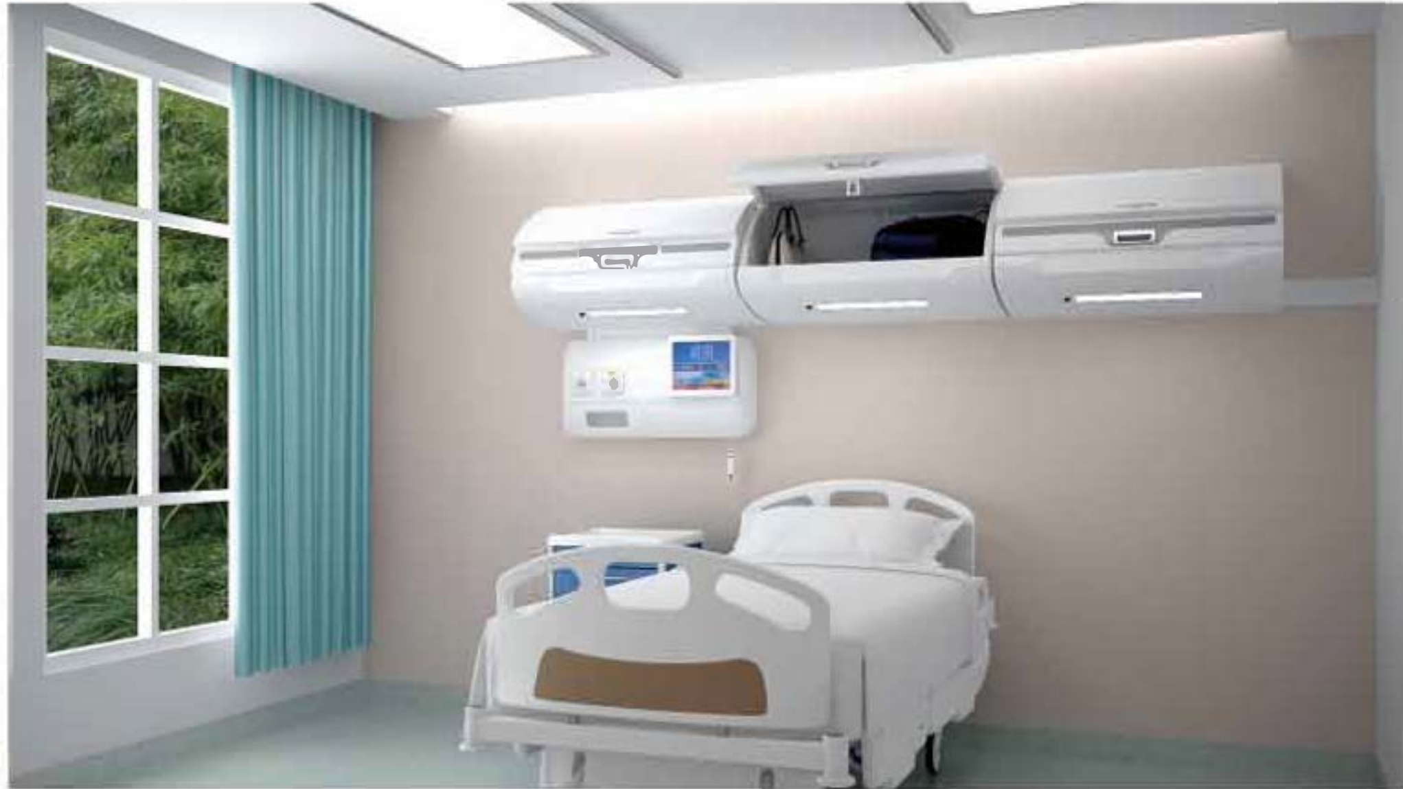
Each bed equip with 3 storage cabinet, 1 set smart integrated panel and digital nurse call system
